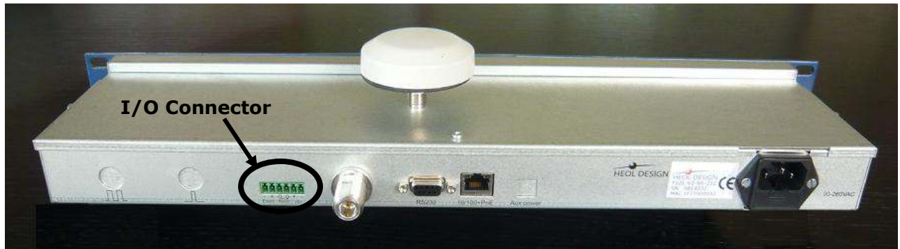
T200 19'' 1U Rack rear view (with 'N' antenna connector)
